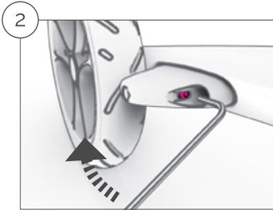
1. Adjust the brake with a 2mm Allen wrench.
