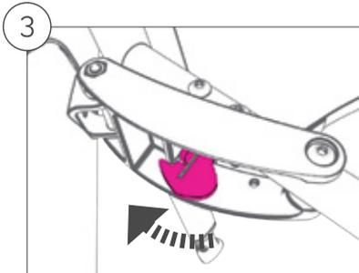
3. If you are in doubt whether the folding mechanism is correctly locked e.g. in a noisy environment, please check that the locking hook under the seat is properly locked into place.
