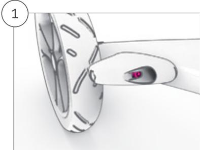
The brake should be adjusted if the brake force applied to the wheel is insufficient (this can occur if the tyres are worn) or the parking brake is difficult to activate (which is most often seen after replacement of a worn down tire). Always set the handle to the desired height before the brake is adjusted as the position may cause a little variation of the brake adjustment.
