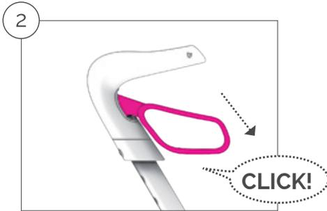
2. The parking brake is activated by pressing the brake lever down until you hear a click sound. Release the parking brake by pulling the brake lever back to the neutral position.
