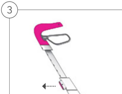
1. Press on the height adjustment button on the frame with one hand while pulling the handle with the other.
