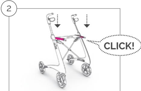
2. Push downwards on the outer rails of the seat in one swift motion, until you hear a significant click from the locking mechanism.
